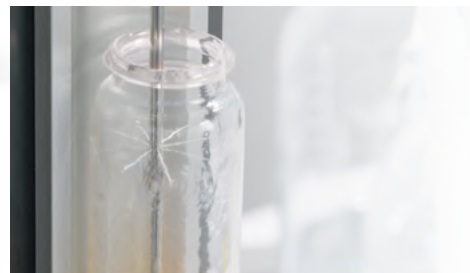
Rinsing of sample vial for quantitative transfer
