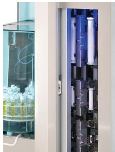
Column carousel is in the forward position for placing the column before processing.
