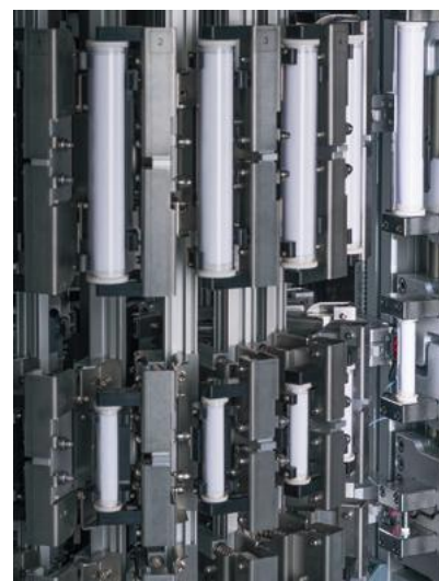
Column carousel is in the rear position with locked columns in the column tower.
