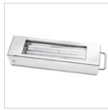
UV-C radiation cassette, protected against water splashes, housing made from stainless steel 1.4301, UV-C emitter with special interior coating of the quartz glass for long service life with low irradiation fall-off, separate electronic ballast, optional insert frame for mounting the cassette (IP 55)
