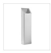
Air disinfection unit for office rooms and doctors' surgeries for wall mounting or as a mobile stand-alone unit, consisting of an air disinfection chamber, fan, micro-filter for pre-cleansing and activated carbon filter, housing made of sheet steel, powder-coated RAL 9010, UV-C emitter with special interior coating of the quartz glass for a long service life with low irradiation fall-off
