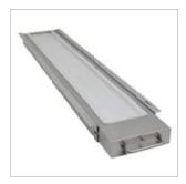
UV-C radiation cassette, protected against water splashes, housing made from stainless steel 1.4301, UV-C emitter with special interior coating of the quartz glass for long service life with low irradiation fall-off, separate electronic ballast (IP 55), optional insert frame for mounting the cassette
