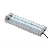
UV-C compact luminaire for air and surface disinfection, specially for deployment in situations with limited space, two UV-C compact emitters, housing made of stainless steel 1.4301, integrated electronic ballast, UV-C emitter with special interior coating of the quartz glass for long service life with low irradiation fall-off
