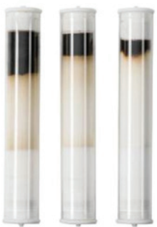
Figure 5 In the silica gel column, fats and other substances will be oxidised. Depending on the fat matrix, the DEXTech™ can process up to 5 g fat fully automatically. Since the column body is made from glass, the user can even optically control the processes. (From right to left: 1 g; 1.5 g; 3 g fat).
