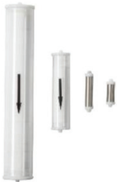
Figure 4 The DEXTech™ system consists of, (from left to right) a silica gel column impregnated with sulphuric acid, a Florisil column, and two carbon columns of different activity.
