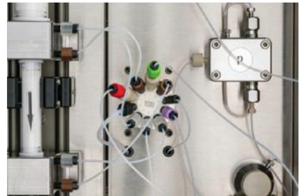
Figure 8 The low solvent consumption is supported by specially constructed, rotatable switching valves with dead space free passages.
