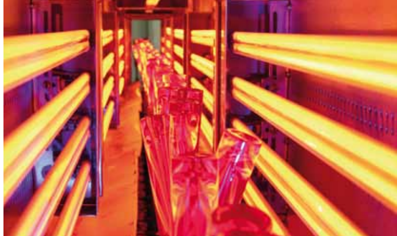
Curing of coatings on glass bottles
