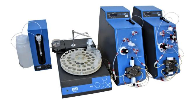
The autosampler **FIAsampler** can accommodate two different sample trays with differing sample volumes. Its integrated dilutor prepares automated dilutions from off-range samples (degree of dilution variable).
