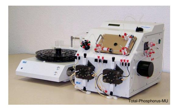
FIAcompact and integrated digestion unit (UV und Thermo) for determination of
